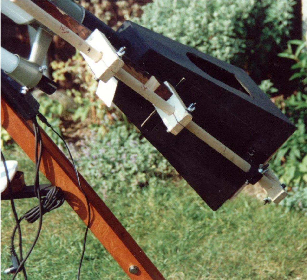
Fig. 4. Fixing the projection box to the telescope
