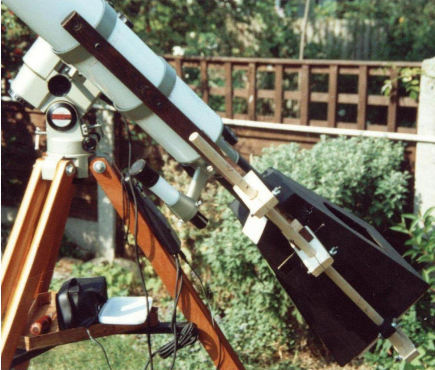
Fig. 5a. Closeup showing observing apertures and rotating screen holder
