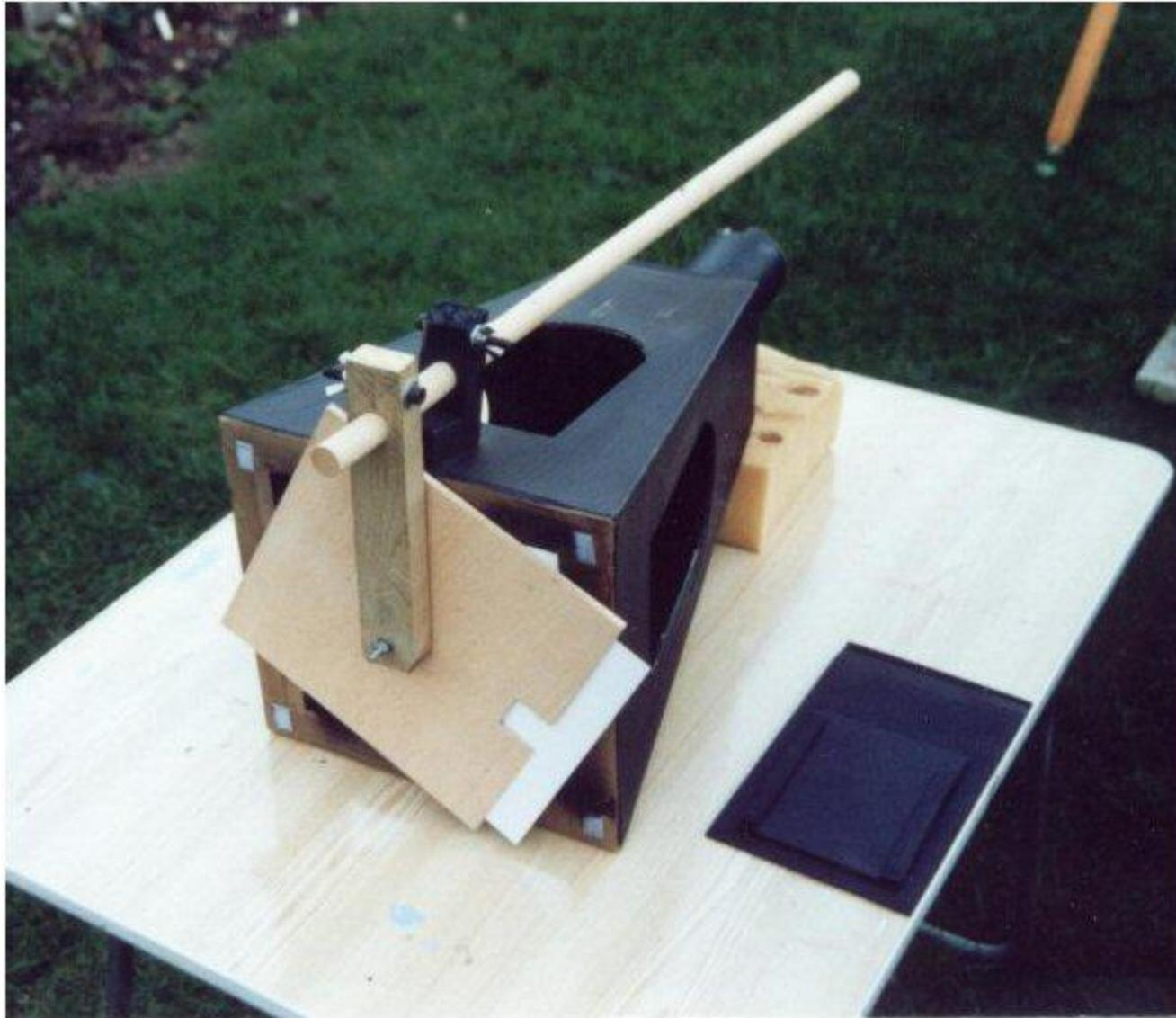
Figure 9. Closeup, showing projection box clamps.
