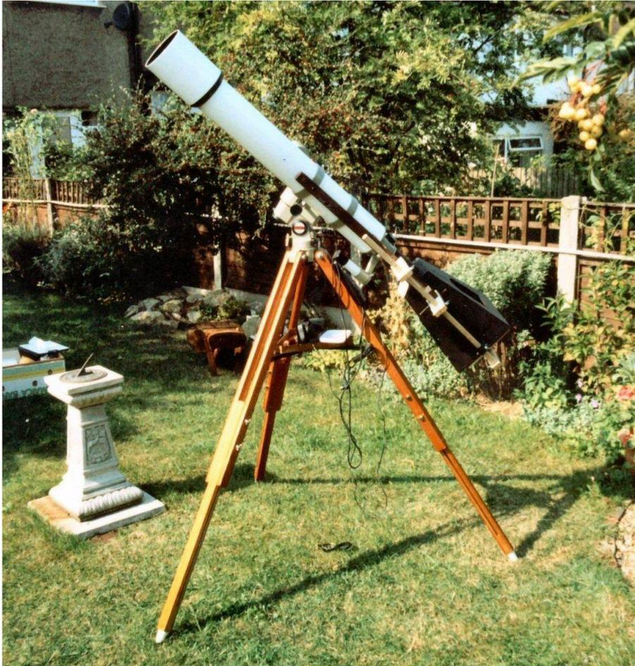
Figure 1a. Vixen GP102M, with solar projection box
