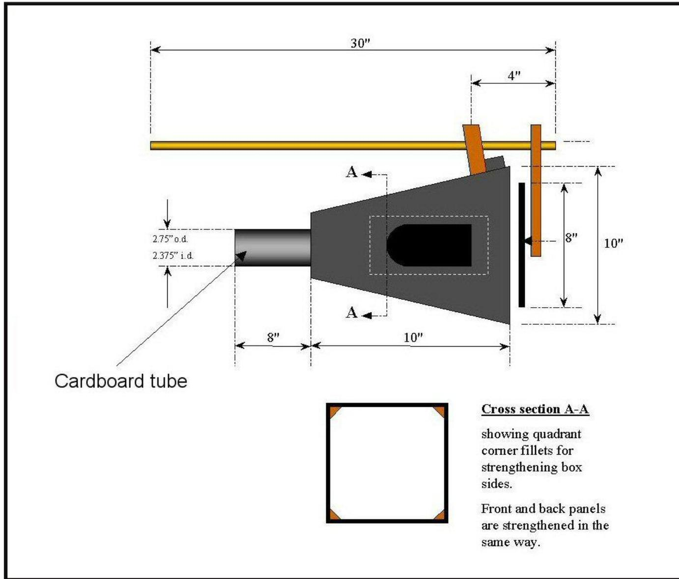
Figure 13. Construction box details
