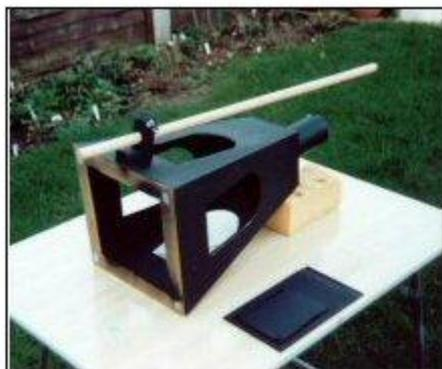
View showing viewing ports. Note Velcro buttons at each corner of back to provide for a translucent screen for public viewing
