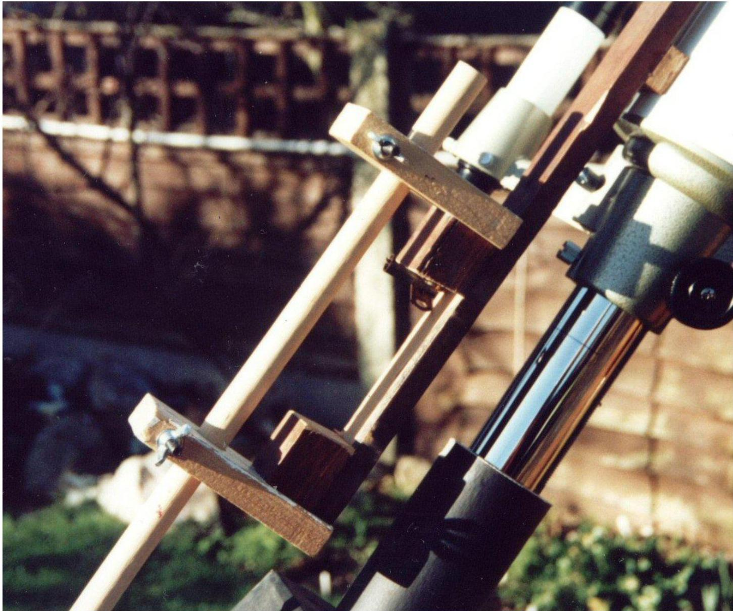
Figure 10. Closeup, showing projection box construction.
