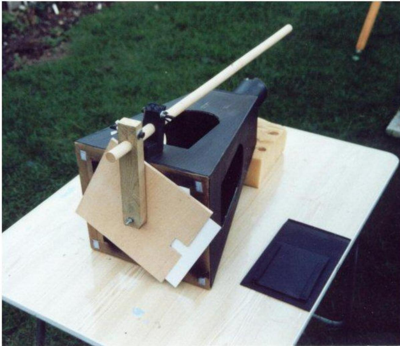
Figure 9. Closeup, showing projection box clamps.
